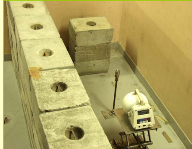
Concrete-moderated neutron field
